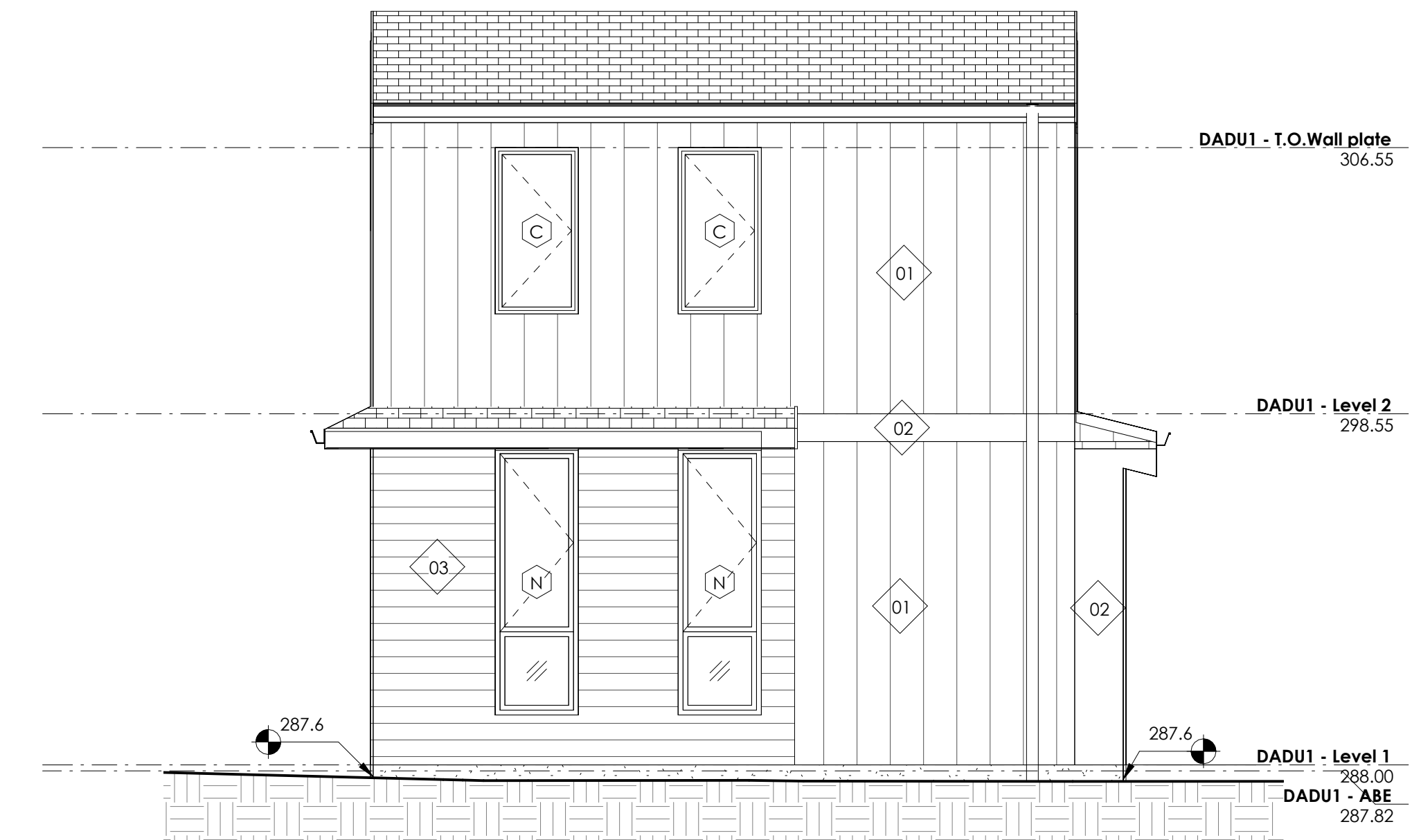
4 DADU ELEVATION - SOUTH SCALE: 1/4" = 1'-0"
